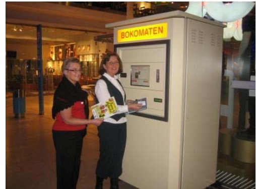
Figure 38: Automated library materials dispensing machine -- shopping mall installation with 400-volume capacity.
